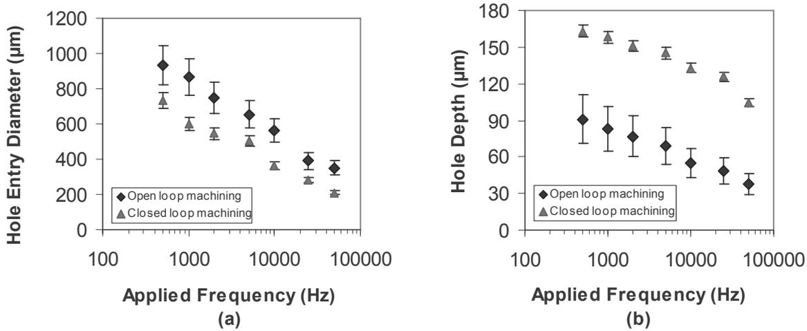
**Fig. 5.** Effect of frequency on (a) diameters and (b) depths for open and closed-loop machining. 30 g/L NaNO<sub>3</sub>, 500 Hz, 16V pp, Ø 0.5mm tool electrode.
