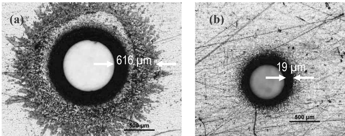
**Fig. 7.** MicroECM hole profile images. Top view of entry hole after ECM'ing with (a) open loop control and (b) closed-loop control.
