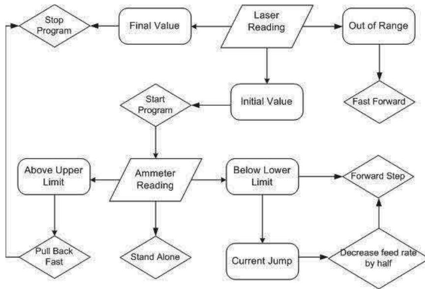
**Fig. 2.** Flow chart of tool electrode position and velocity control.
