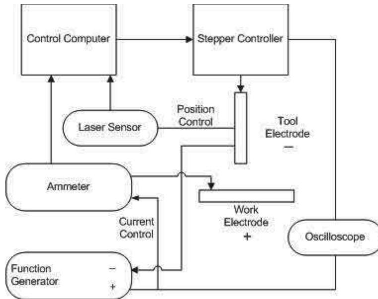
**Fig. 1.** Current and position controlled setup.
