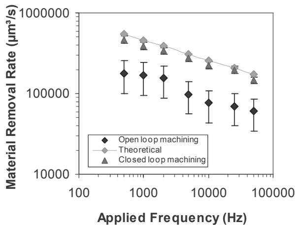
**Fig. 6.** Material removal rate with frequency. 30 g/L NaNO<sub>3</sub>, 500 Hz, 16V pp, Ø 0.5mm tool electrode.
