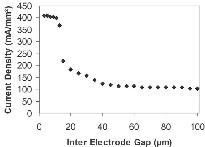
**Fig. 4.** Effect of electrode gap on ECM current density. 30 g/L  $\text{NaNO}_3$ , 500 Hz, 16V pp.
