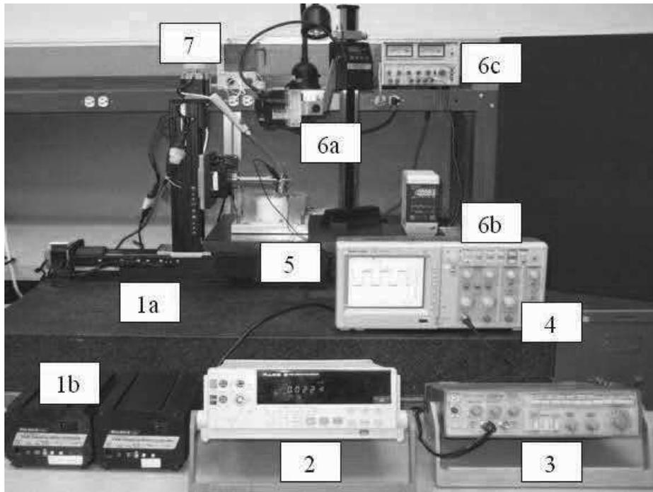
**Fig. 3.** Closed-loop microECM setup. (1a) stepper motors, (1b) motor controller, (2) ammeter, (3) function generator, (4) oscilloscope, (5) ECM cell, (6a) laser displacement sensor, (6b) laser controller and display, (6c) power source for laser unit, (7) electrolyte tank and jet pump.
